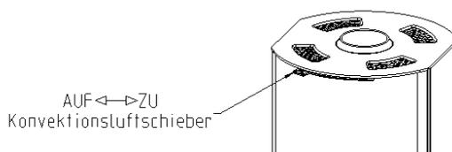
Our hint: while the fire still burns let the convection air outlets open; close them after the fire has burnt down in order to reach a steady heat emission.
